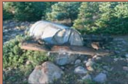
Stockrollers compacted earthen-filled dams. The roller was made on site from corrugated metal and concrete hauled up to the lakes.
