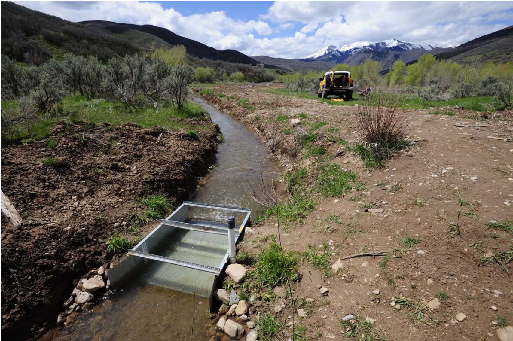
Figure 2. Photograph of ramp flume #1 with the stilling well attached.
