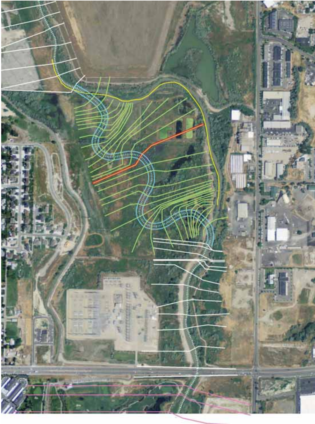
Figure 6. Aerial image showing the location of HEC-RAS cross sections for Alternatives 4 and 5. The cross section location highlighted in red was used to generate the cross section plot shown in Figure 7.
