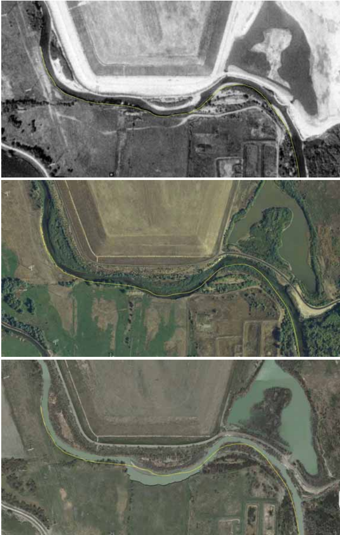
Figure 2. Channel erosion in the Big Bend area, south of the Sharon Steel cleanup site. The top image shows the channel as pictured in the 1990's Ortho Maps, including a trace of the southern edge of the active channel (yellow line). The middle and bottom images show the same area in 2003 and 2012, respectively. Note the bank erosion and channel widening that has occurred, mostly after the 2003 DDPR was completed.
